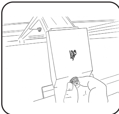
Place K9 clamp in position and hand tighten. This should be done to all clamps provided.
