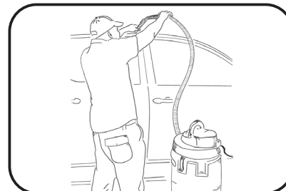
Lift out rail and vacuum out all loose particles.
